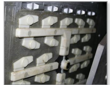
An FDM split pattern bolted to a matchplate blank.
