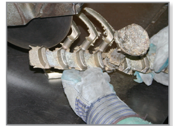
Cut off gates and risers from cast part.
