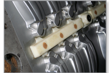
A matchplate with an interchangeable FDM gate and runner system.
